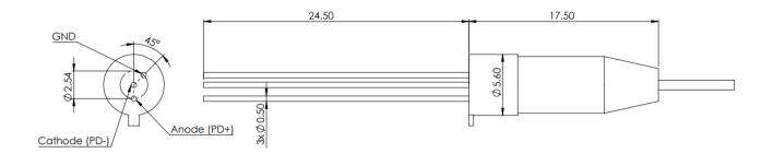
Standard Package for Infrared Band. For other wavelength band, size may vary due to special detector configurations.
